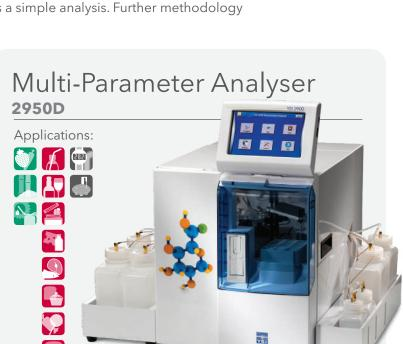
Using YSI's highly accurate biosensor technology, the 2950D may measure up to 6 compatible chemistries. These include glucose, lactate, sucrose, galactose and lactose within the dairy industry with applications varying from lactose in cheese/milk, lactate in silage, probiotic production and many more.
